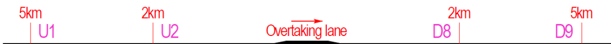
Figure 3.10: Traffic counter locations and nomenclature either side of the surveyed passing lane sites
