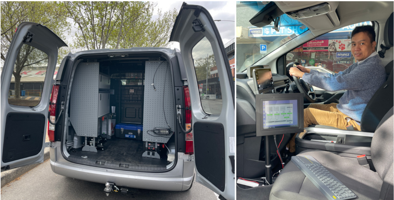
Calibration of the new TCA test vehicle is being finalised. The vehicle is used to test hardware and devices submitted for type approval.
