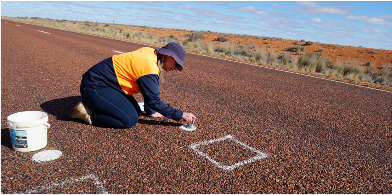
The latest inspection of sprayed seal trial sites in Coober Pedy indicate polymer modified binders are aging better than unmodified bitumen.
