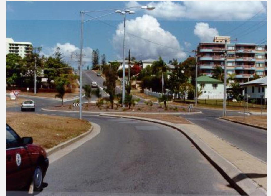
Example of reverse radius curve approach. Source: MRWA (2015)
