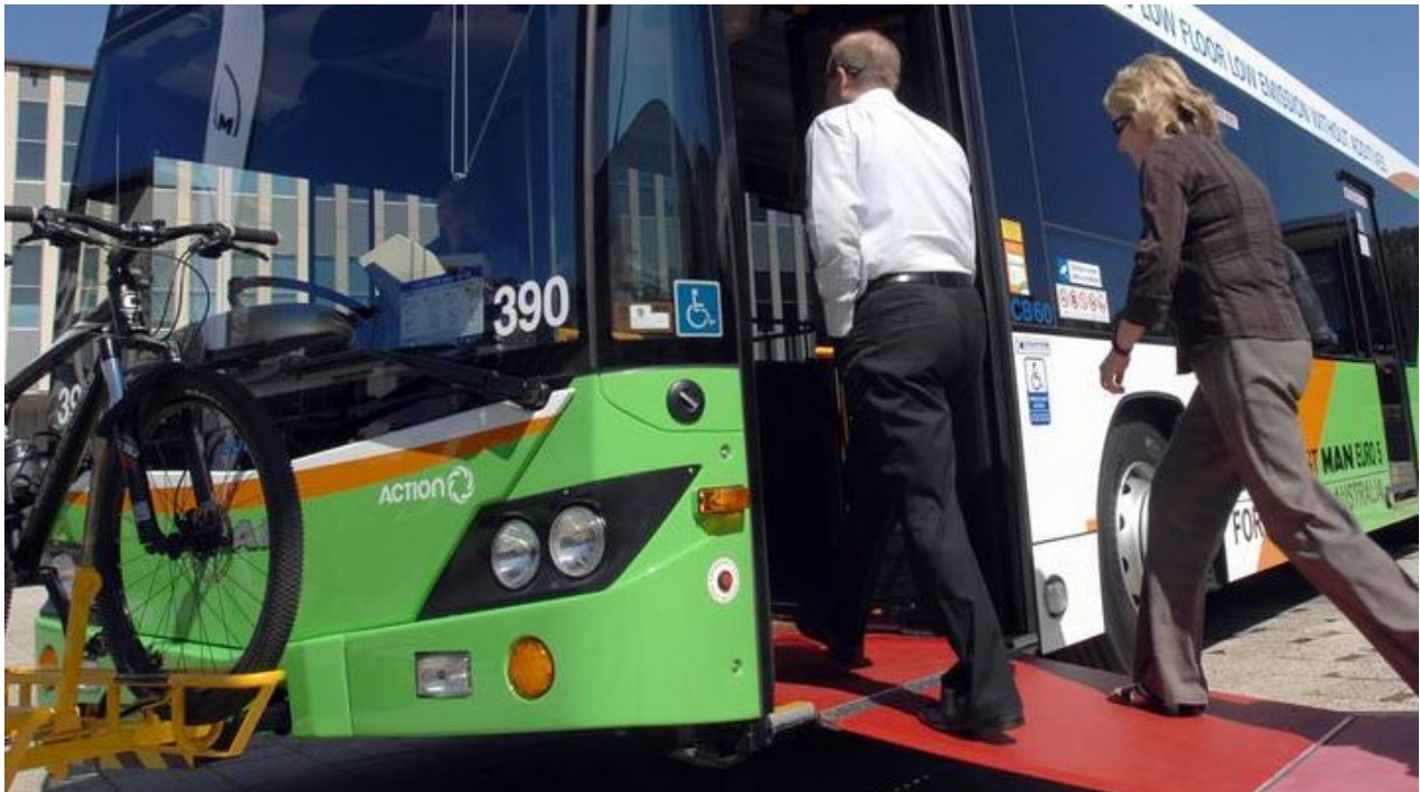
Figure 7.43: Bike racks on buses, Canberra
