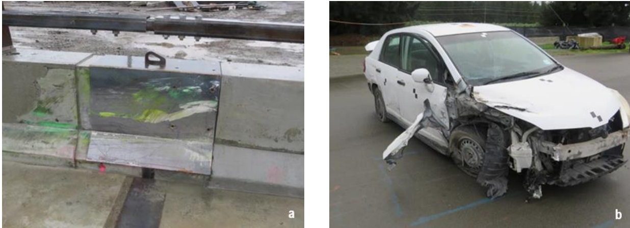
Figure 10.2: Results of crash test 5-10 on (a) barrier system (b) test vehicle
