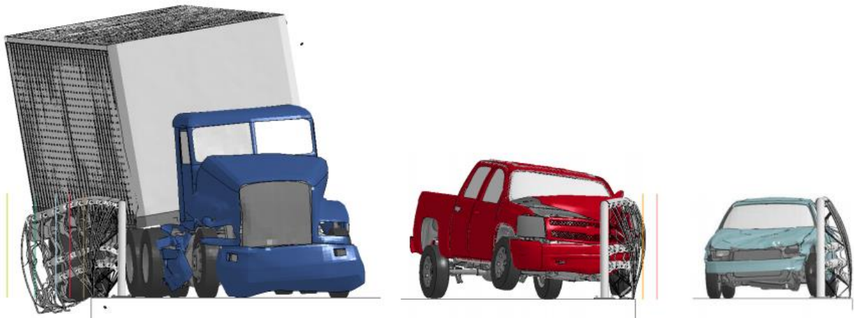
Figure 1.2: Simulation of Dolre TL5 design according to the Manual for Assessing Safety Hardware (MASH)
