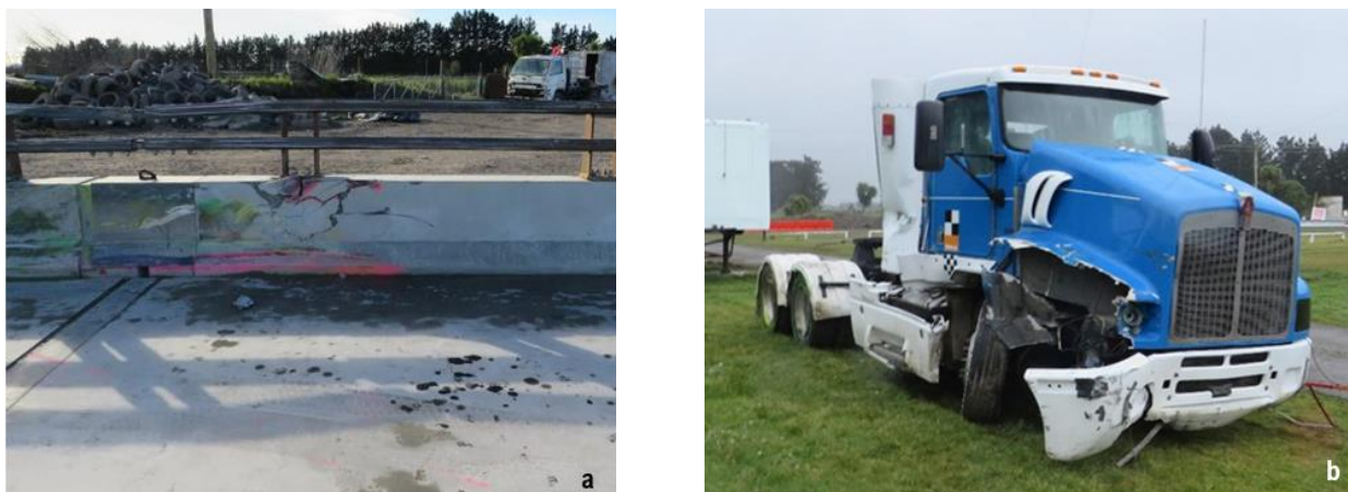
Figure 10.4: Results of crash test 5-12 on (a) barrier system (b) test vehicle
