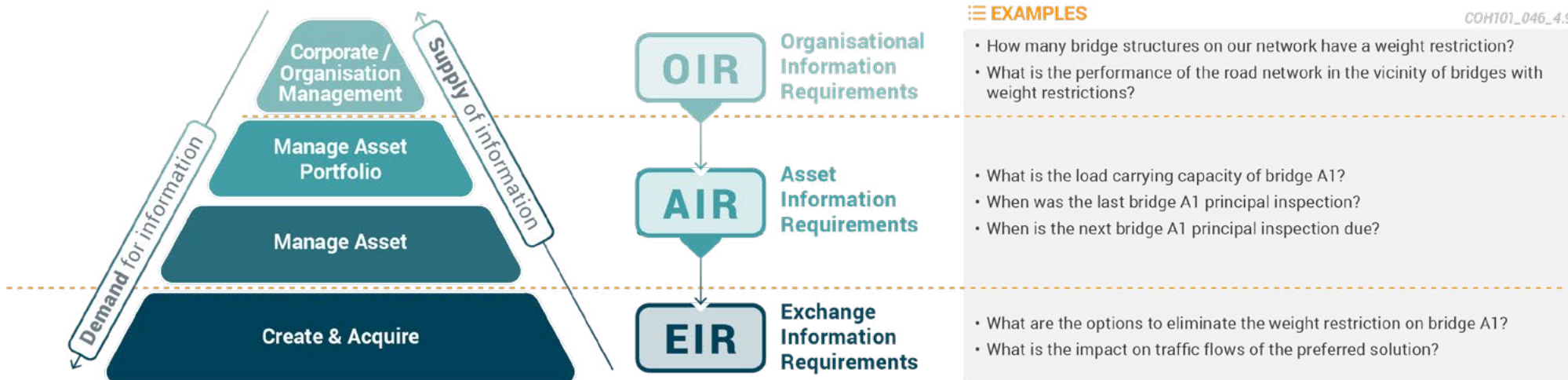
Figure 4.8 - The relationship of Information Requirements managed across operations, maintenance and within projects.
