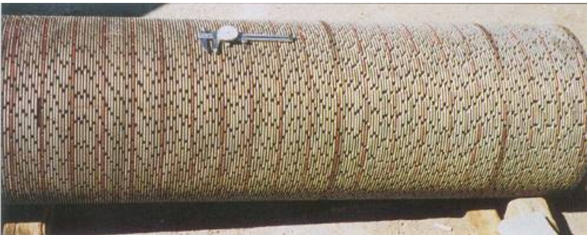
Figure 9.4: Diamond grinding head for concrete surface texture correction
