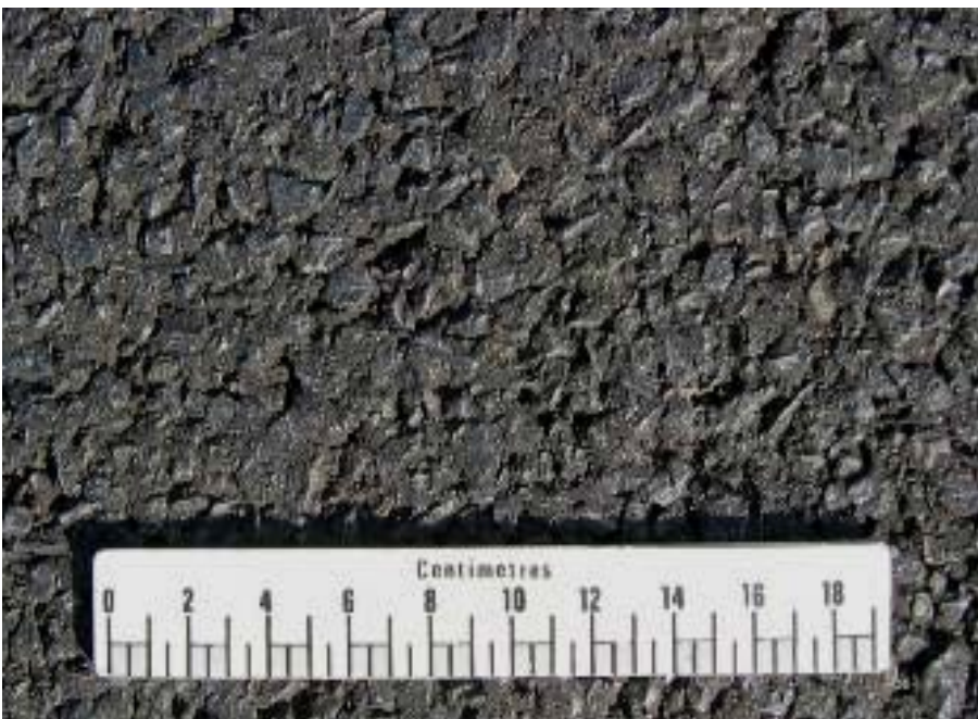
Figure 2.7: Stone mastic asphalt
