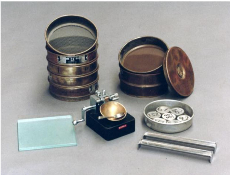
Figure A 1: Equipment used to determine grading and plasticity index of fines
