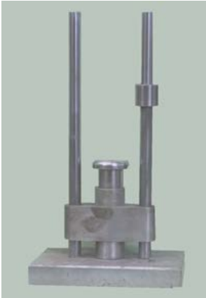
Figure A 4: Rigden device used in AS 1141.17 to assess packing behaviour of fillers
