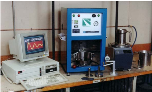
Figure B 4: Gyropac and ancillary equipment with computer attached to a PC to automatically record the compaction process
