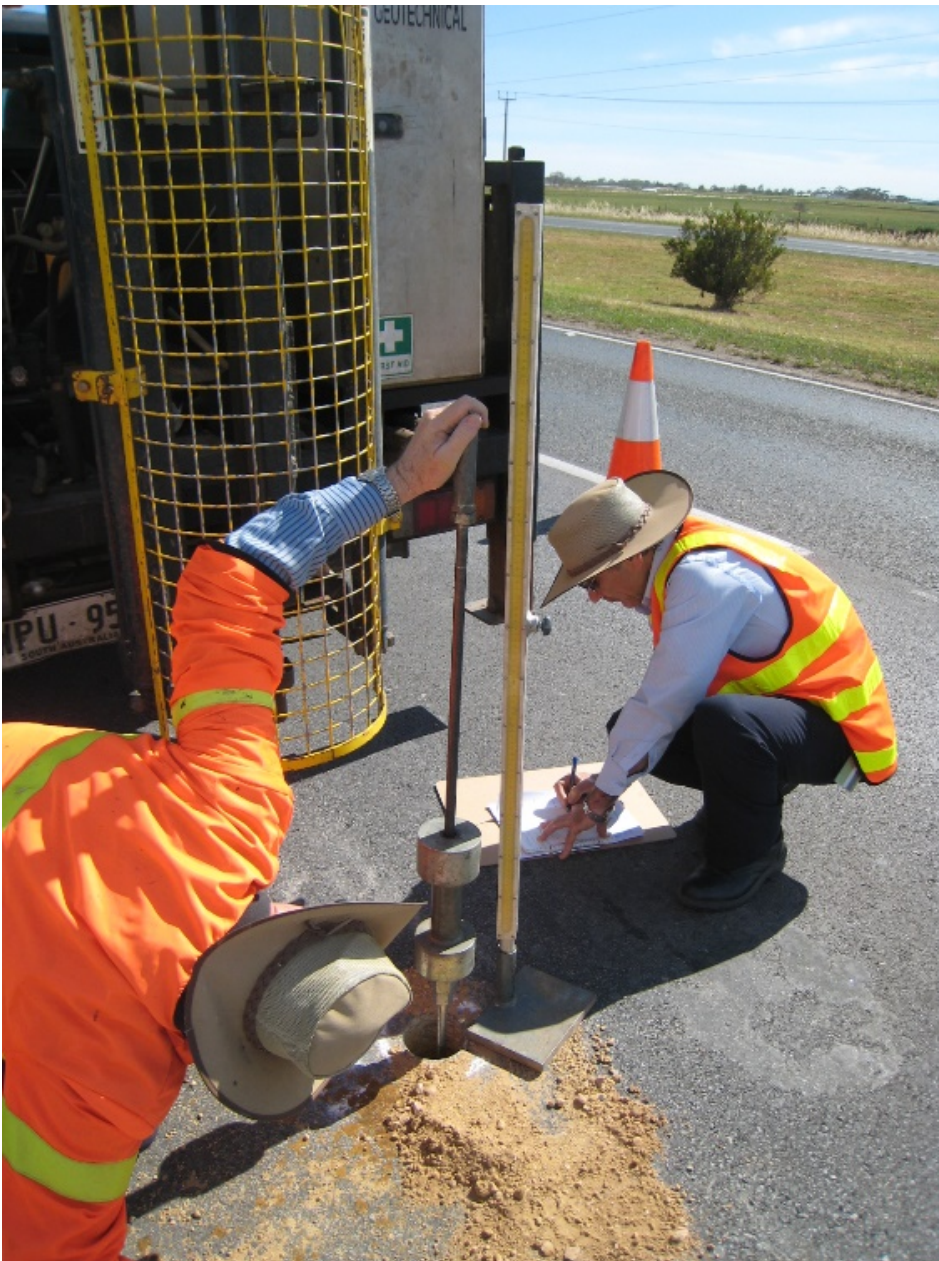
Figure 5.2: Dynamic cone penetrometer
