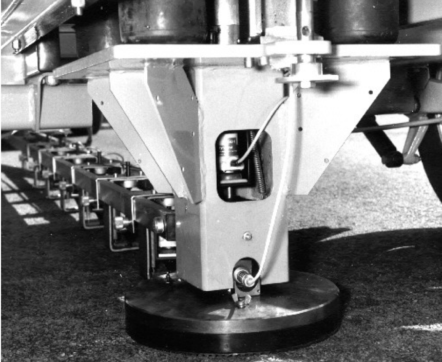
Figure 4.21: FWD loading plate and geophones to measure pavement response to load
