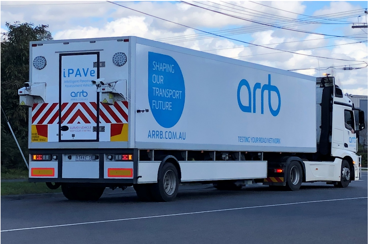
Figure 4.22: Traffic speed deflectometer
