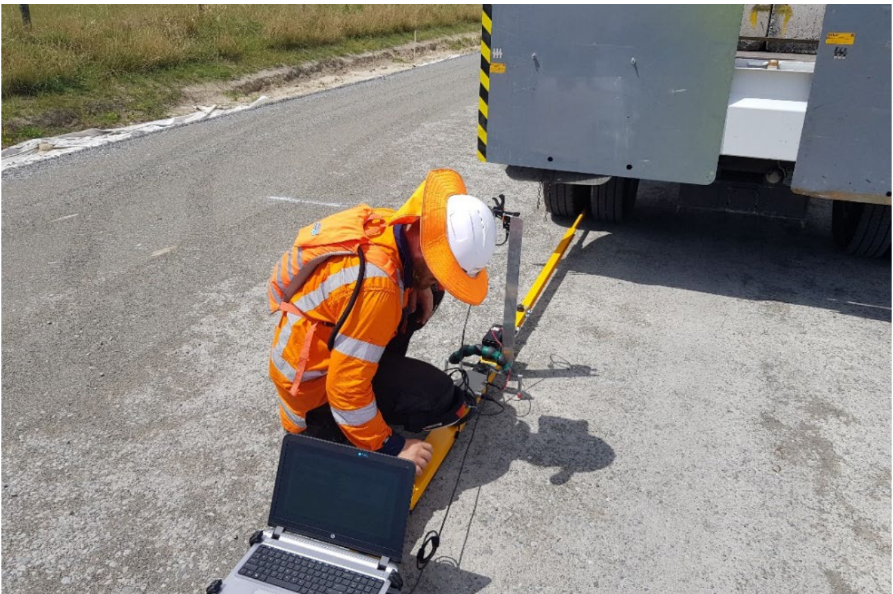
Figure 4.17: Benkelman Beam with load truck and data logger to record measured deflection bowl
