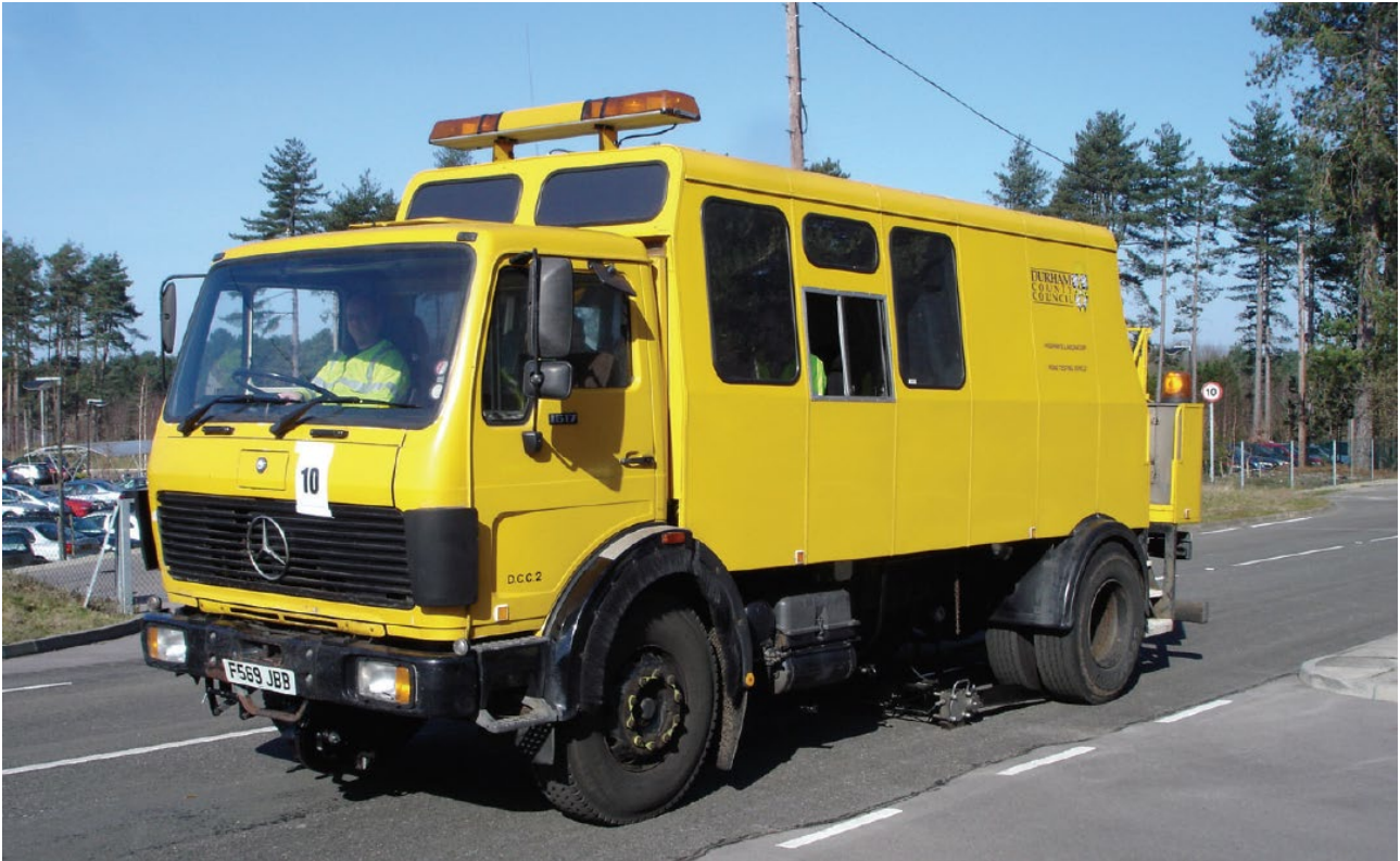
Figure 4.18: Host truck with loaded rear axle and deflection measurement sled in front of rear axle
