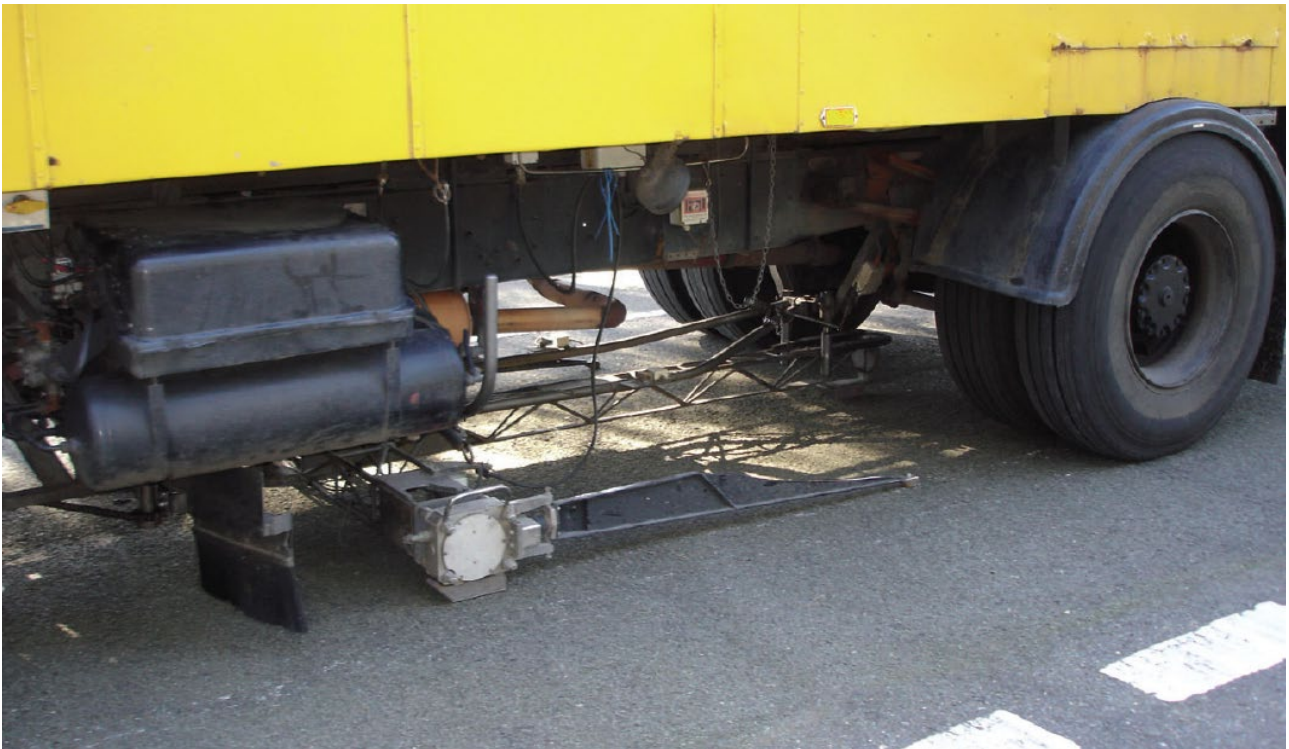
Figure 4.19: Deflectograph with measurement beam shortly after starting a deflection bowl measurement
