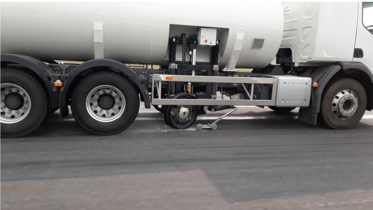
Figure 4.12: Instrumented test wheel
