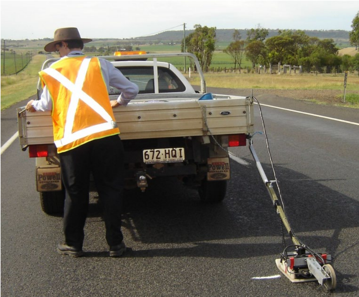
Figure 4.15: Example of a ground-coupled antenna with distance-measuring wheel set-up behind a vehicle
