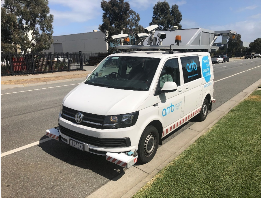
Figure 4.3: Network survey vehicle complete with Inertial laser profilometer
