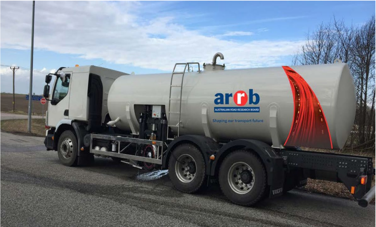
Figure 4.11: Truck-mounted skid resistance tester
