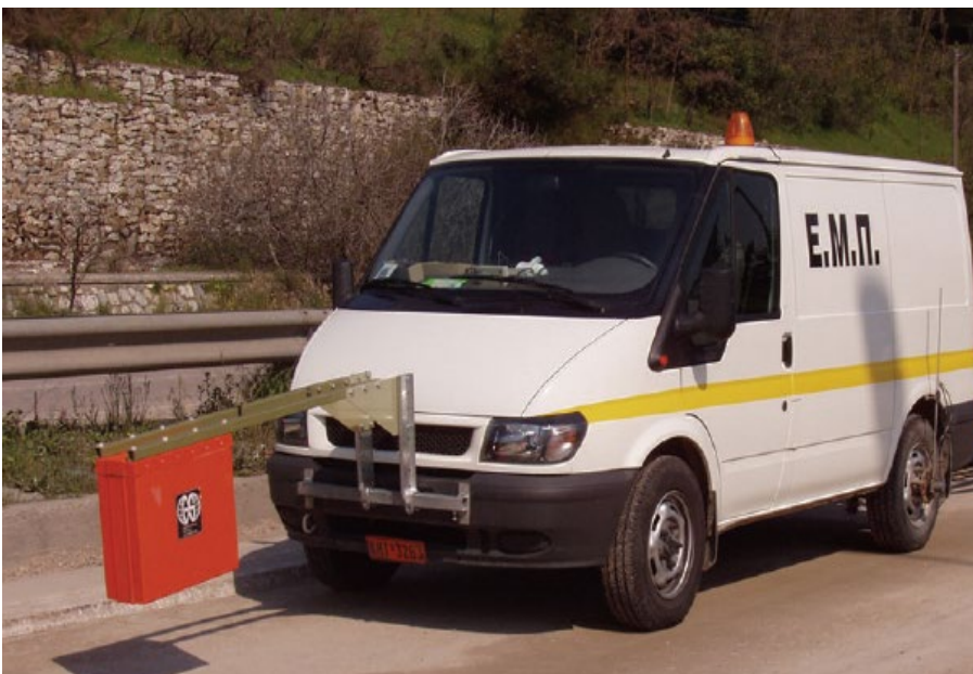
Figure 4.16: Example of an air-coupled antenna mounted on the front of a vehicle
