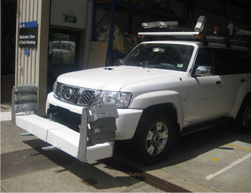
Figure 4.6: An example of a multi-laser profilometer
