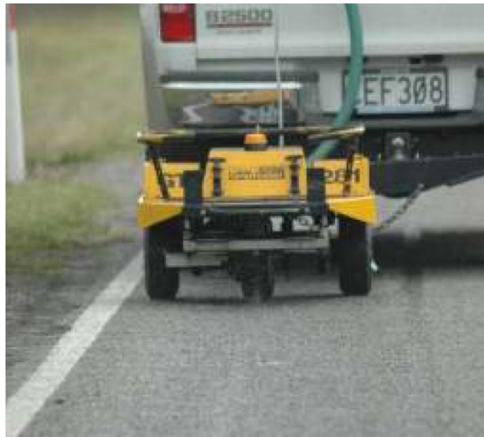
Grip tester in operation
