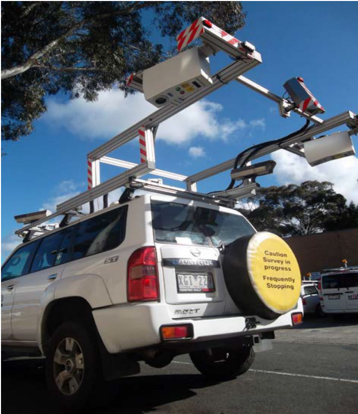
Figure 4.10: LCMS automated crack survey device
