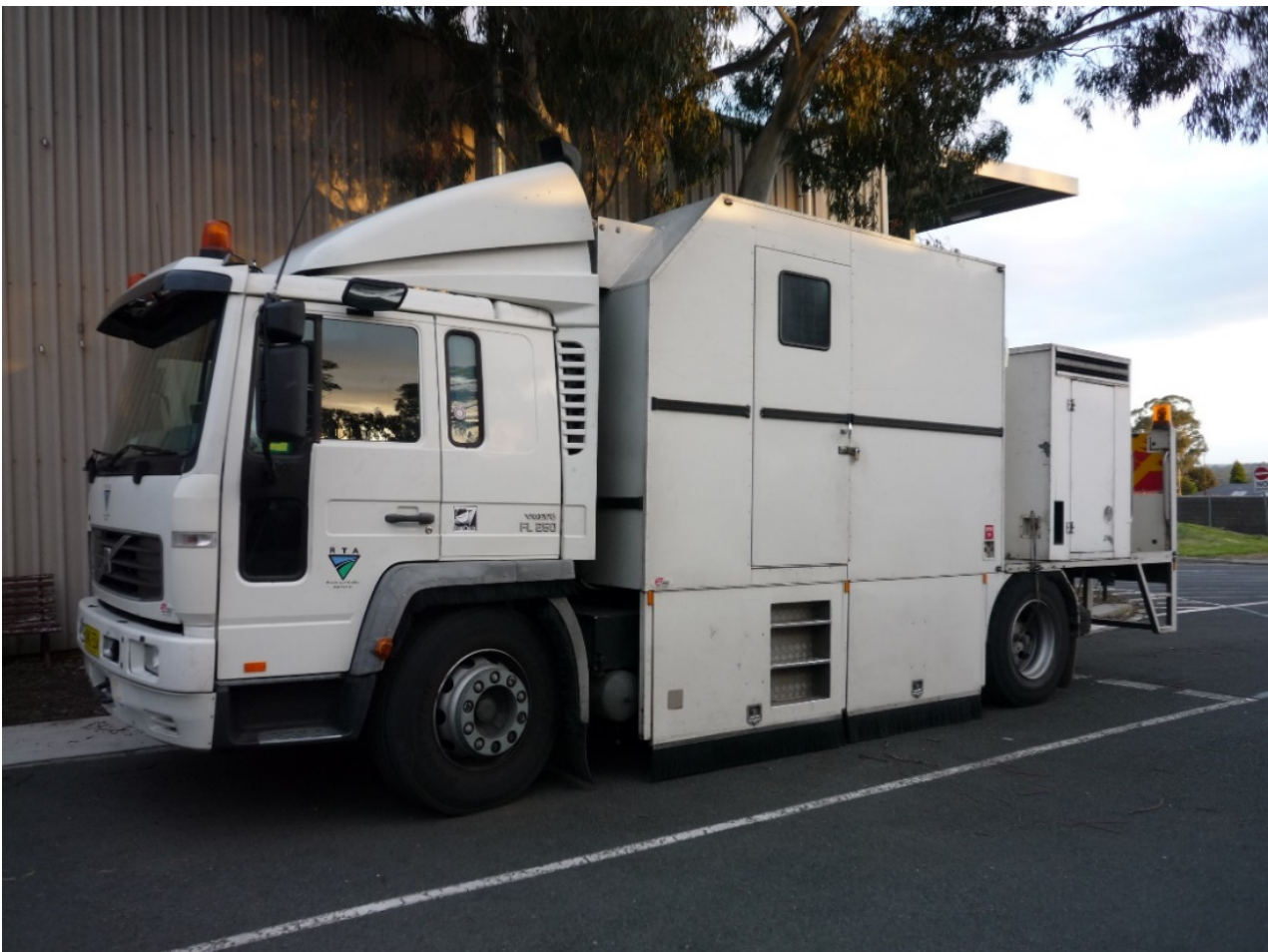
Figure 4.9: Roads and Maritime RoadCrack automated crack survey device
