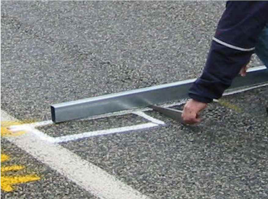
Figure 4.5: Straightedge and wedge manual rut depth measurement
