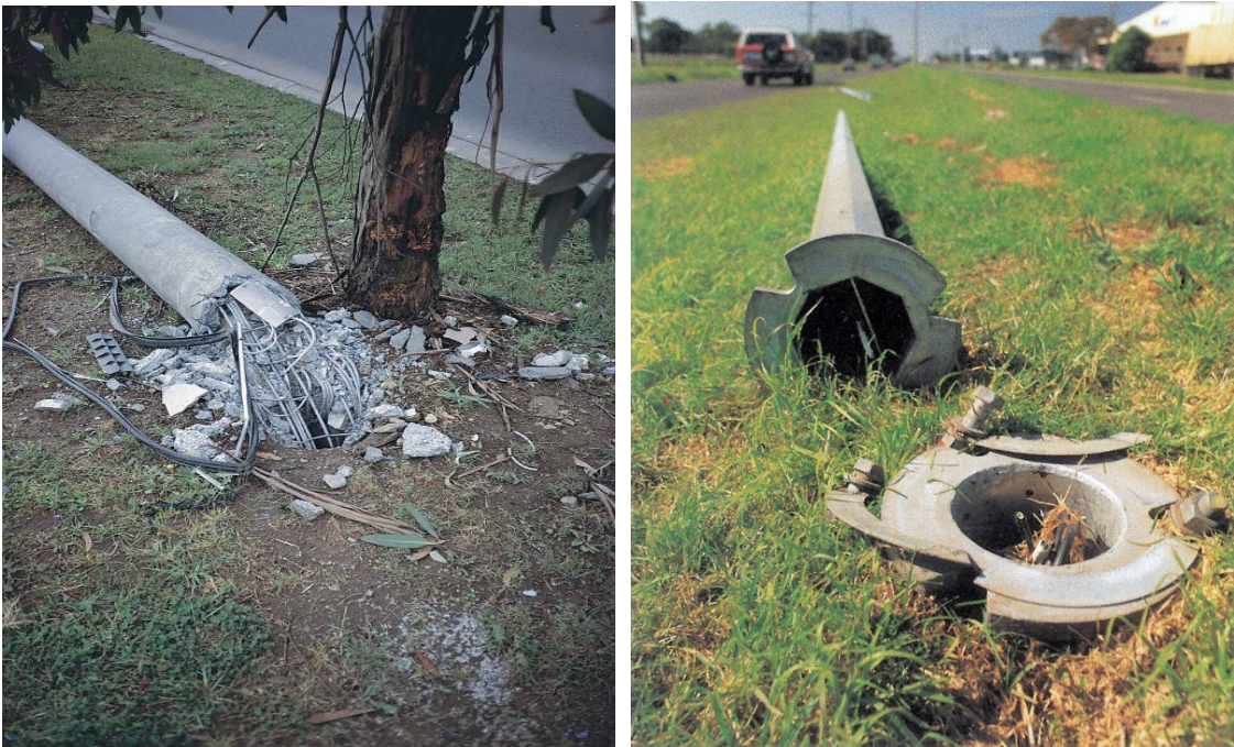
Figure 6.16: Concrete pole (left) and slip-base pole (right)
