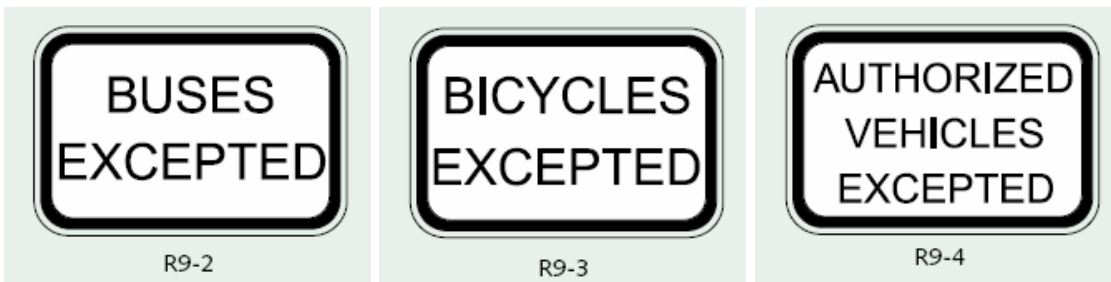
Figure 8.51: Supplementary plates excepting special vehicles from turn bans
