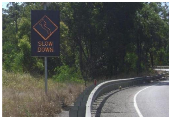
Figure 5.13: Examples of vehicle activated signs on an approach to a curve in the form of a CMS and VMS application
