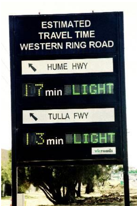
Figure 5.5: Trip condition sign
