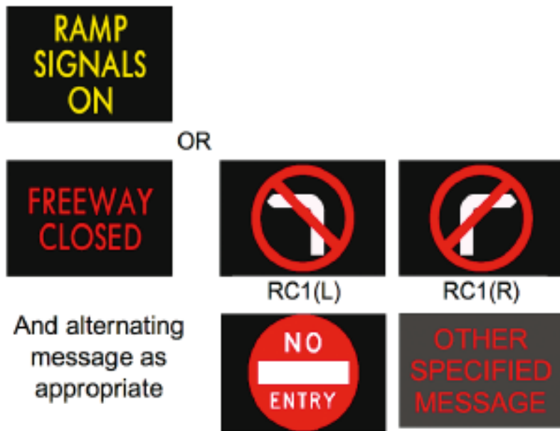
Figure 5.8: Example of electronic ramp control sign messages
