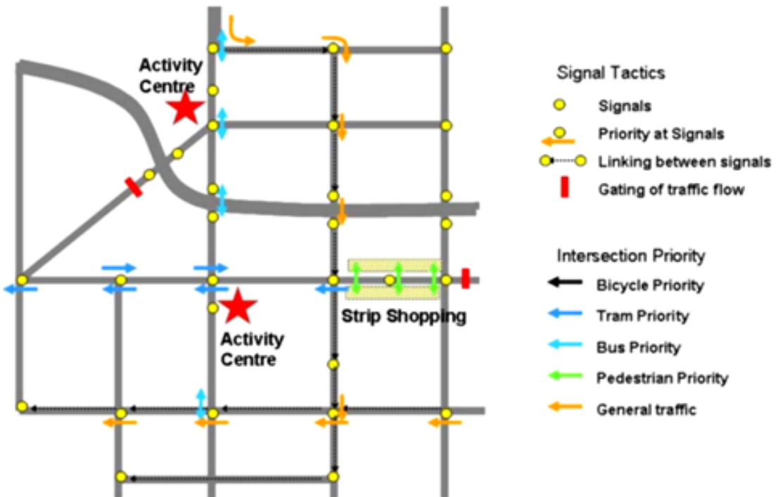
Figure 4.6: Signal operation plan for a region
