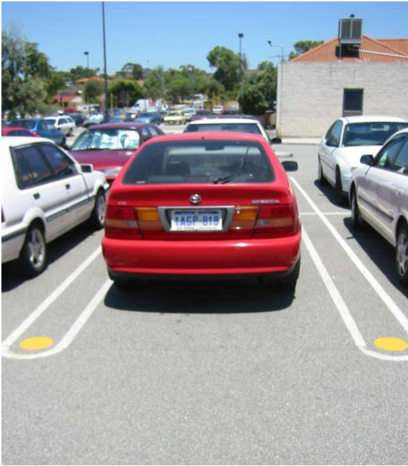
Figure 7.5: Example illustrating good off-street parking bay delineation practice
