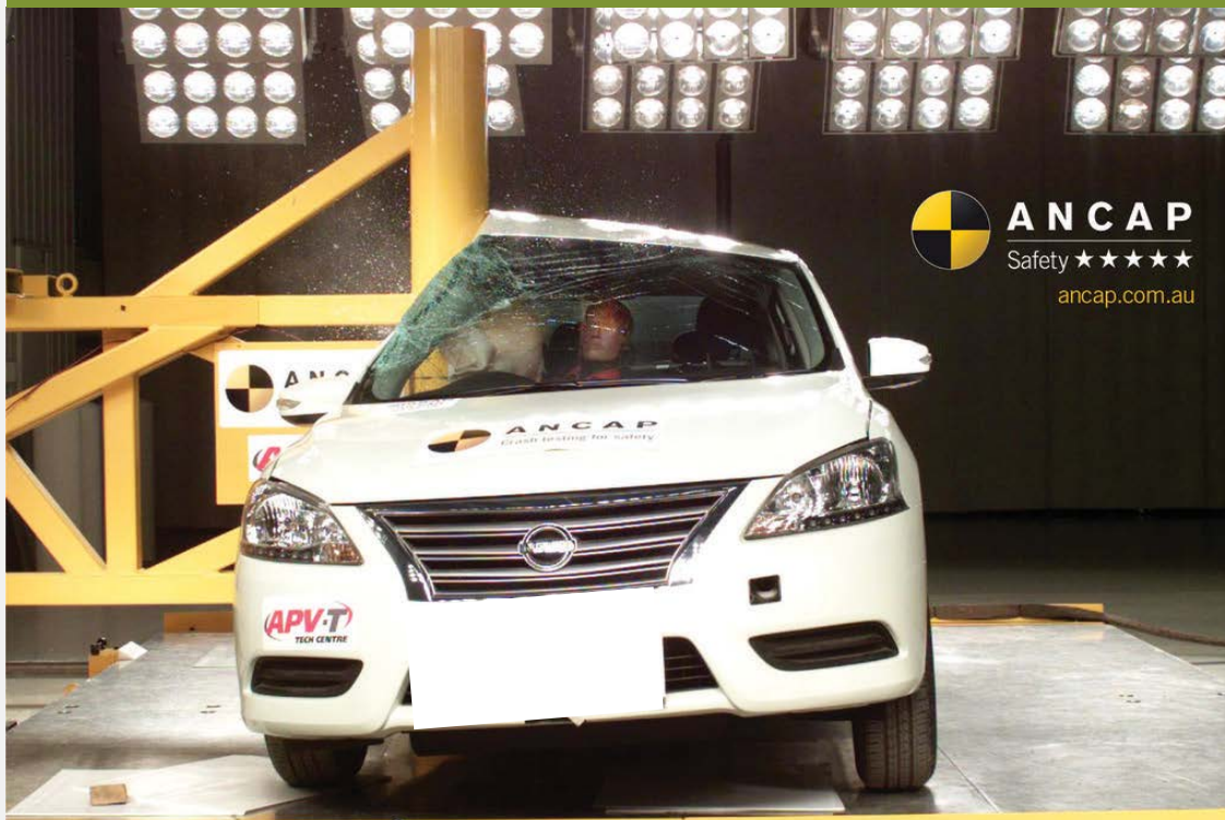
Pole side impact in lab at 29km/h
