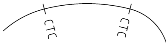
BROKEN-BACK CURVES ( Joined by large radius curve )
